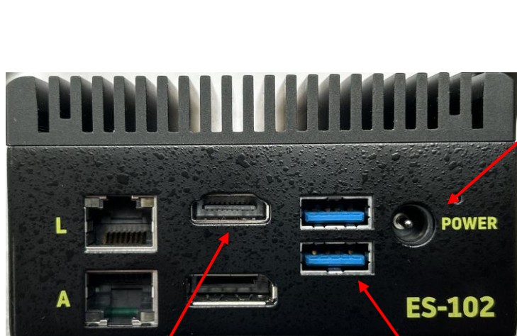
HDMI (Monitor) port and USB ports
